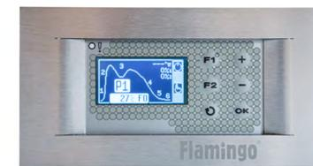
It controls the air intake dampers, which regulate the burn process. Thanks to the fluent regulation is the burning clean, optimal and prolongs the burn time. The automatic control unit uses the values from the flue gas sensor and that is why the automatization process is very precise.
